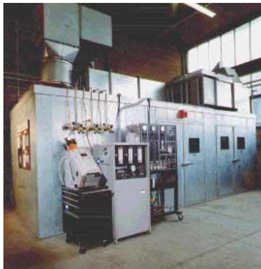
Figure 6: A spray booth set up inside an existing workshop (Picture courtesy TWI)
